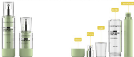
The bottle is easy to replace the inner bottle when screwing open the bottom. The inner bottle's material can be PCR which is more environmental friendly. With fresh and simple appearance, the refillable design will be more popular for the different brands.
